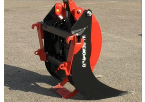
The grip claw is easily and safely stored when the gripper arm is completely closed, functioning as a kickstand.
