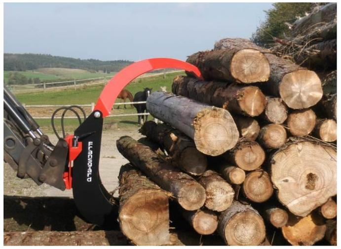
The large opening height of the upper arm and long forks allows grasping a large volume of timber.
