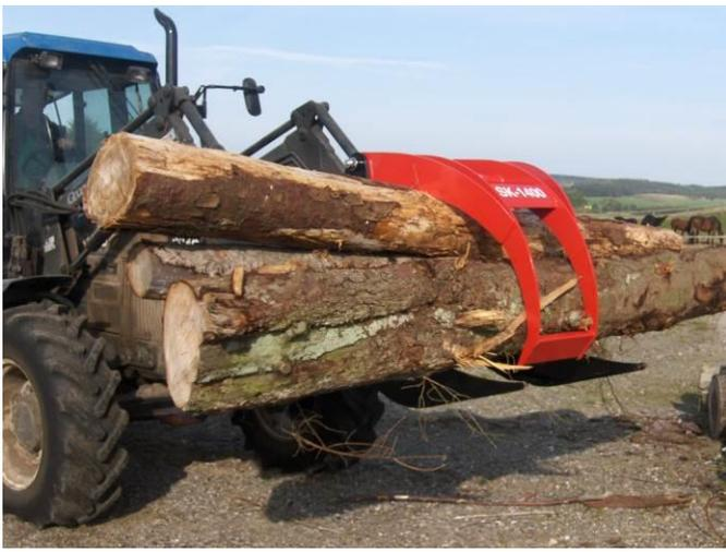
The upper arm securely holds the timber against the long forks, even if the middle grip is not tight
